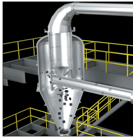
Figure 3. When the material is conveyed to the large separating chamber, air pressure is dropped to allow the material to fall into the chamber below.
